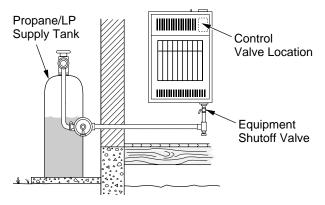
Figure 16 - Checking Gas Joints for Propane/LP Gas
